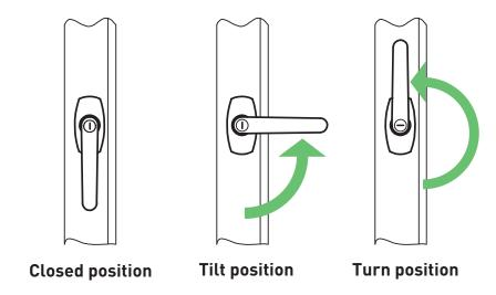
**Please note:** The above operation is for "Tilt before Turn" or "Tilt First" gear. "Turn before Tilt" or "Turn First" gear is also available although less common. If this is fitted the handle position shown above for the Tilt Position & Turn Position would be reversed.
